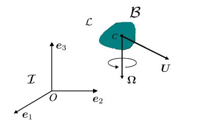
The motion of  $\mathcal{L}$  is described from a frame,  $\mathcal{S} = \{C, e'_i\}$ , attached to  $\mathcal{B}$
