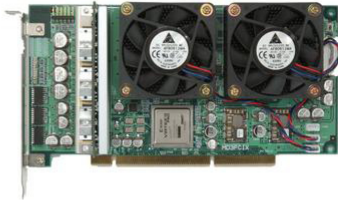
FIG. 3.1 Hardware accelerator: MDGRAPE-3 PCI-X board
