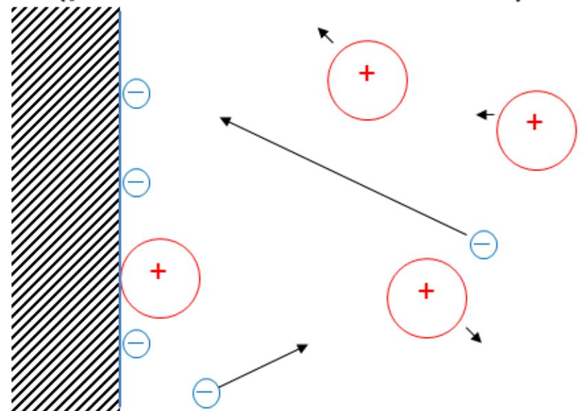
Wall is negatively charged due to the flux difference, causing potential gradient in the space
