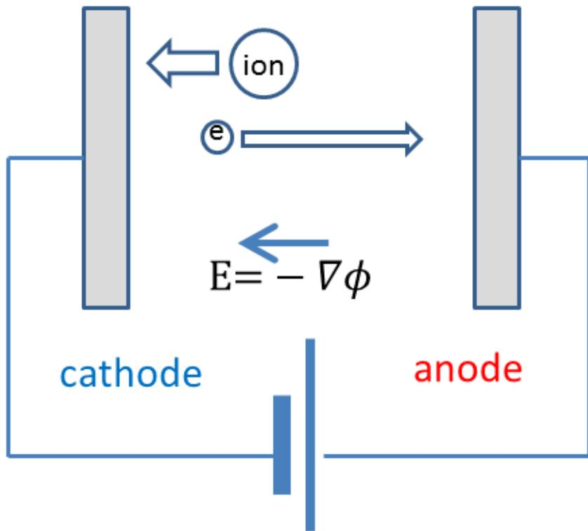
Voltage difference accelerates ions toward **cathode**, and electrons toward **anode**.
