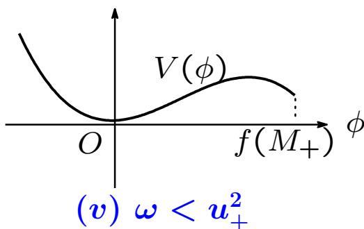
$$f(\tilde{\rho}) := \frac{u_+^2}{2} \left(1 - \frac{1}{\tilde{\rho}^2}\right) - K \log \tilde{\rho}, \quad V(\tilde{\phi}) := \int_0^{\tilde{\phi}} [e^\eta - f^{-1}(\eta)] d\eta. \quad \begin{pmatrix} \text{Sagdeev} \\ \text{potential} \end{pmatrix}$$
